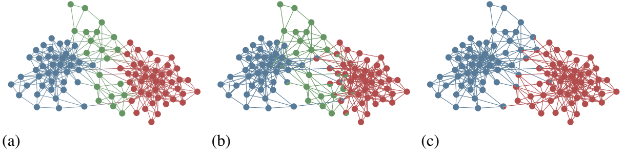
Figure 10. Network of co-purchase of books about US politics [66], with groups inferred using (a) the non-overlapping DC-SBM, with description length \Sigma \approx 1,938 bits, (b) the overlapping SBM with description length \Sigma \approx 1,931 bits and (c) the overlapping SBM forcing only B = 2 groups, with description length \Sigma \approx 1,946 bits.
